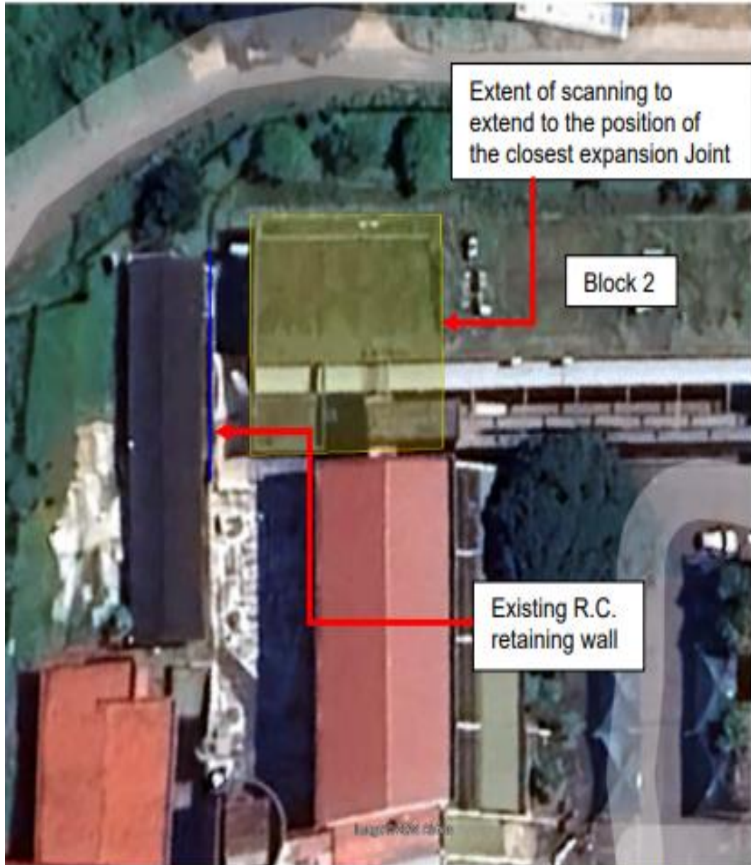
Figure 1: Building to be scanned (Yellow) and R.C. retaining wall (Blue)
